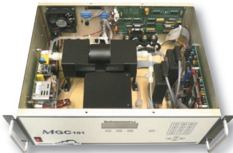
MGC 101 - internal view
